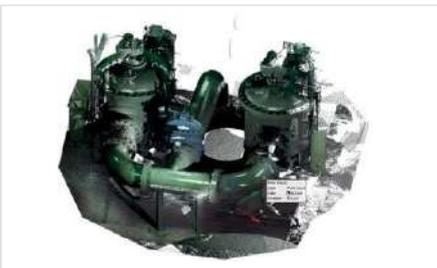
**Point Cloud Processing** – nanoCAD opens and views 3D point cloud files captured by laser scanners in LAS, BIN, PTS, PTX, PCD, and XYZ formats. This means that users can work with extremely large point clouds of one billion points and more. Users have access to point cloud metadata and can work with points cloud as if they were vector objects, such as changing insertion points, scaling, 3D mirroring, embedding 3D models, and taking sections plane of them.
